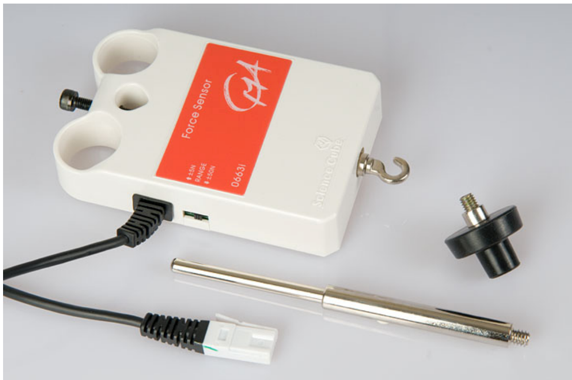
Figure 1. The Force sensor with two ranges \pm 5 N and \pm 50 N
