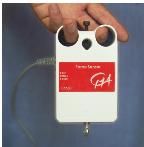
Figure 3. The Force sensor can be hold by hand or mounted on a ring stand.
