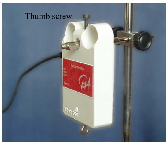
Figure 3. The Force sensor can be hold by hand or mounted on a ring stand.
